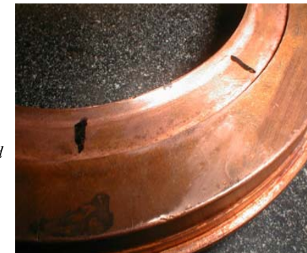
This copper mask gets damaged on the edges. Carr's laser weld the damage and machine the diameter to size.
