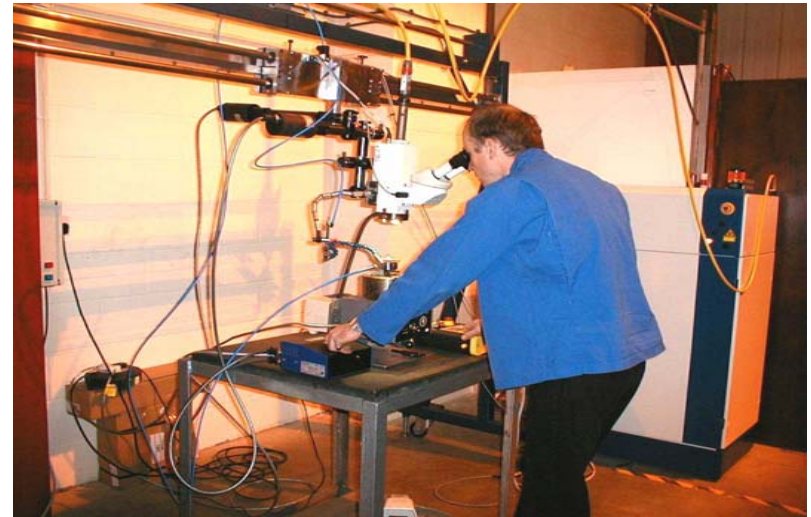
The new laser 5 system at Carr's for large tools and deep penetrating welds.
