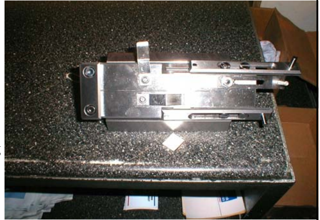
Purpose built jig for laser welded parts
