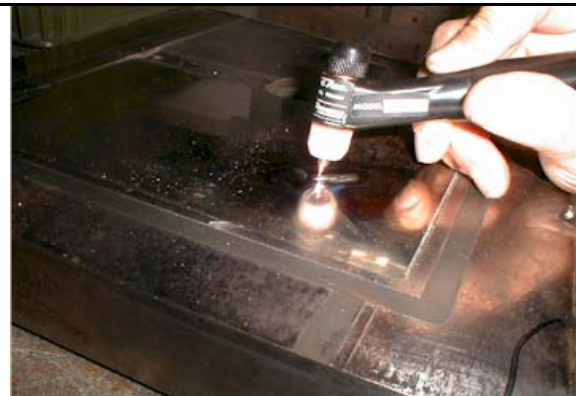
Plasma welding onto stavax tool, where water ways were cracked.
