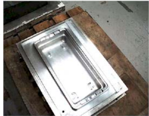
Aluminium tool had weld porosity, Carr's welded & dressed.
