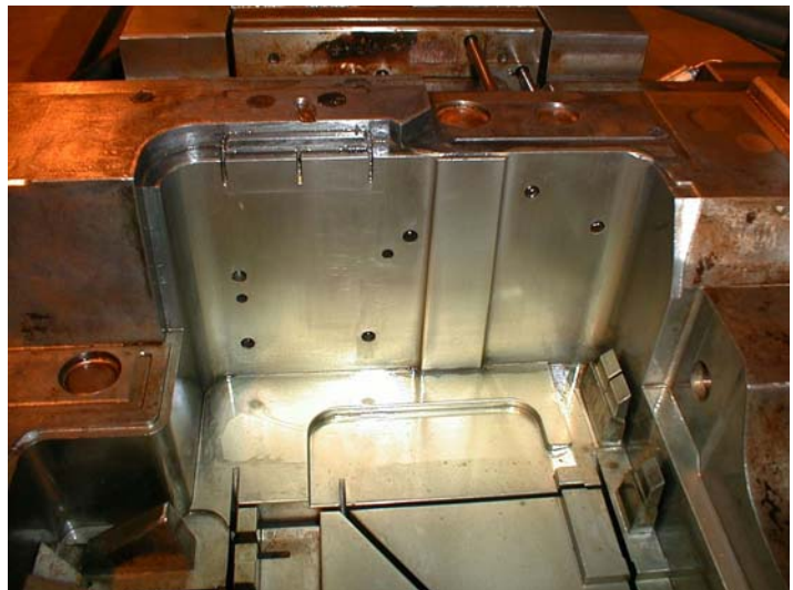
Automotive Battery tray cavity repaired at Carr's.
