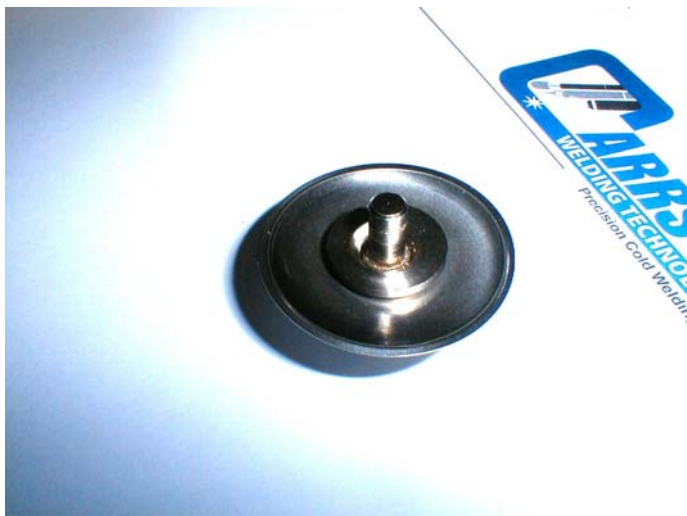
Stainless steel spring valve assembly laser welded together.
