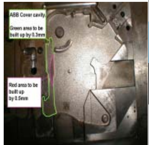
The cavity needed modifying by a controlled thickness.
