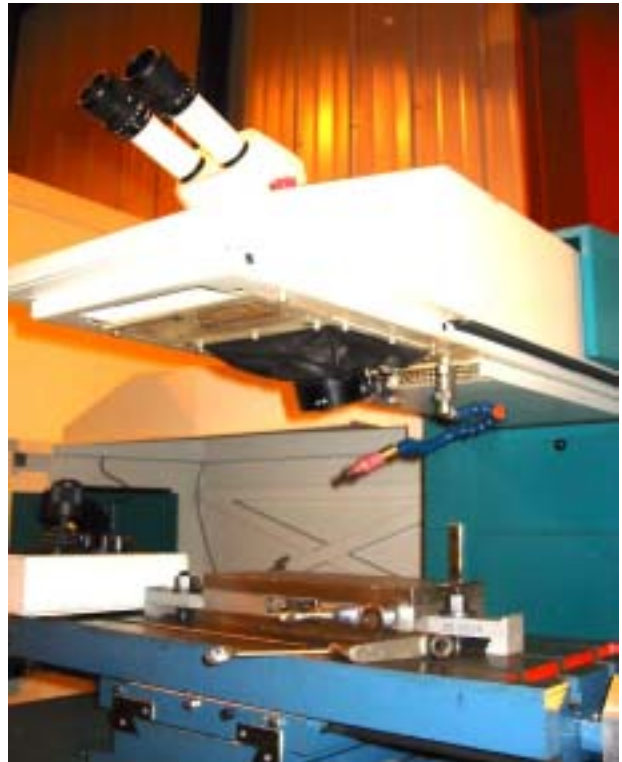
Carr's new laser welder with angled head allowing better access to the welded area.
