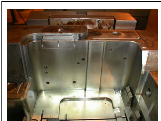
P20 cavity required score marks repairing from the plastic flashing into bores. The wall was cold welded and dressed by hand. The bores were cold welded and re-cut.
